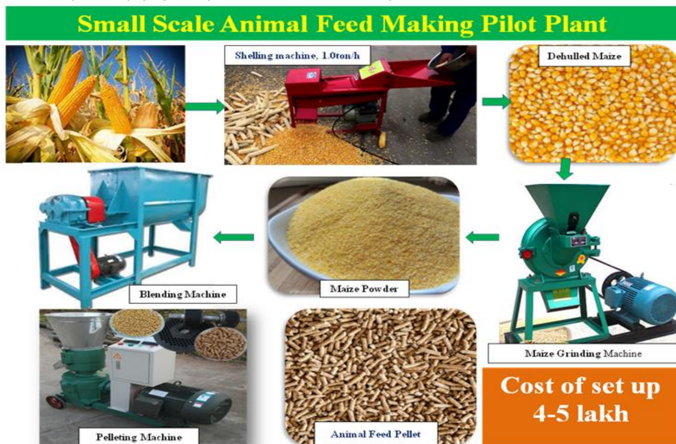
Figure 8. Equipment related to complete animal feed manufacturing plant (Singh et al. 2022b) 37
