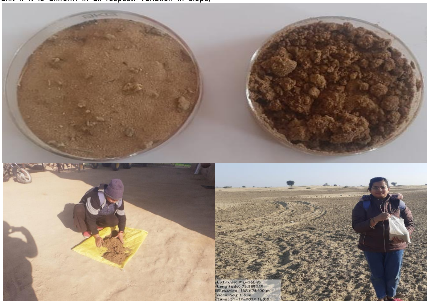
Plate 1. Soil samples collection from various study sites subsequent with coning and quartering method. Samples can be drawn satisfactorily with any one of hand implements namely, soil tube auger, screw type auger, post hole auger, spade and khurpi
